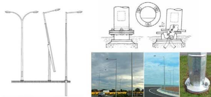
Figura 21: Stâlpi de tip “rupere de la bază” (Source: Department of infrastructure, Energy and Resources: Road Hazard Management Guide, Tasmania, 2014)
